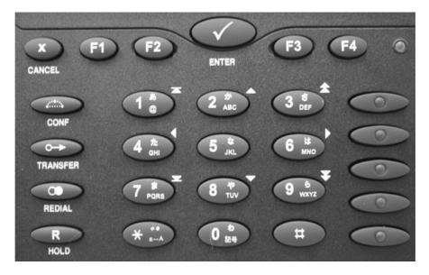
The MENU key is used to invoke the main menu. To cancel actions or input, the CANCEL key can be used. The ENTER key confirms actions, selections and inputs.
